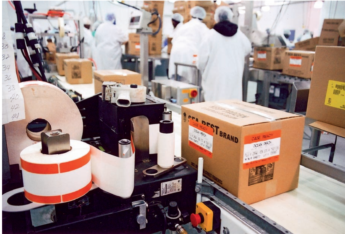
Sealed cases convey over an in-motion checkweigher that relays information to a PC. This data is then sent to a print-and-apply labeler downstream, above, that applies front and side labels to the cases.
